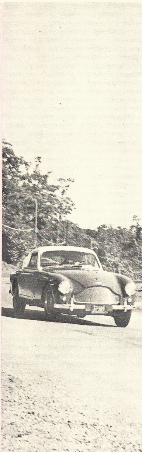
Nearly on limit, front suspension is still able to cope with surface irregularities despite large roll angle.
